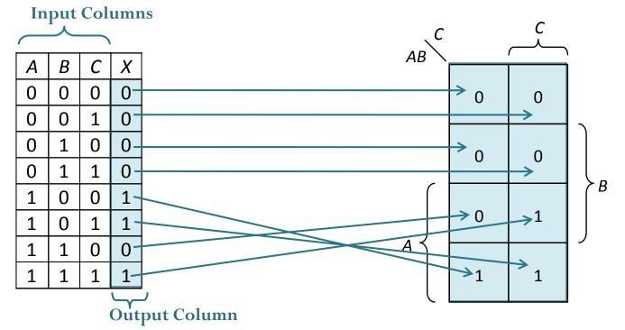
It can be difficult (especially for large K-map) to remember which cell in K-map corresponds to a particular row in the truth table.
